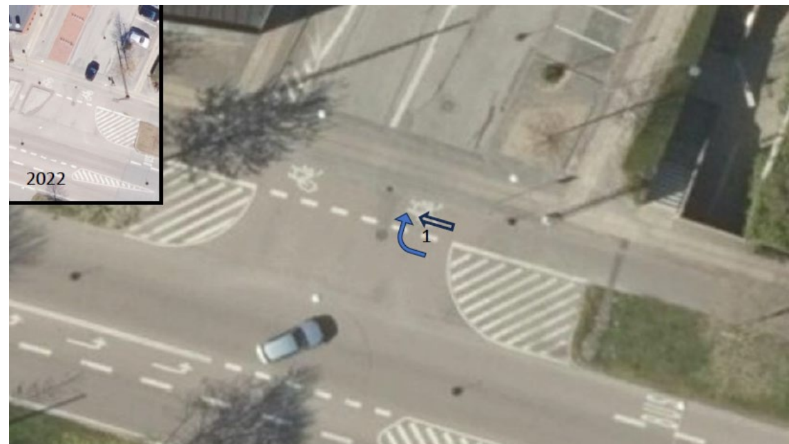
After improvement (photo 2017): continuous sidewalk and improved markings give narrow design which slows down turning cars: 1 material accident of this type in 6 years (2014-2019)
